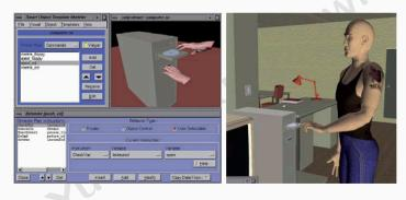
– The semantic information in the smart object is used by the virtual characters to perform actions on/or with the object, such as grasping it, moving it, and operating it (e.g., a machine or an elevator).
